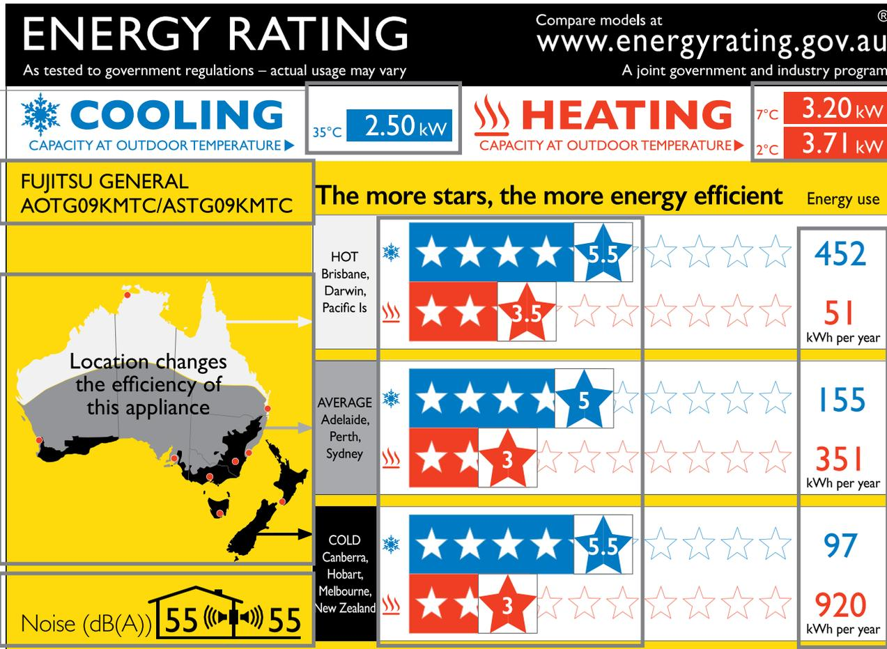
If the temperature outside is hot (35°C), then the Heat Pump/Air Conditioner can provide 2.50kW of cooling.
